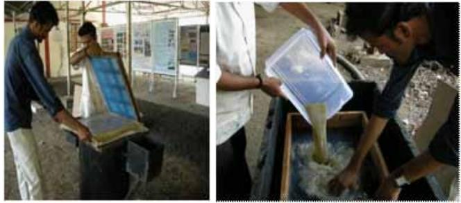
shake it so that the pulp uniformly settles over the mesh. Take the mesh out of the tank as the water drain through it. The process of depositing formed paper over the wet cloth is called couching. Thickness of the paper can be adjusted by changing the quantity of pulp used for making paper in the mesh.
