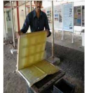
Take a piece of Gada cloth that has sufficient size to cover the entire outer surface of the vat. Place a neat & wrinkle free Gada cloth over the mesh (that now has the pulp) in such a way that no gaps, folding or water bubbles occur in the pulp formed on the cloth. For each sheet of pulp use different layers of cloths and place it one over the other. Once the sheets formed on the cloth or stacked together then place it in the screw pressing to remove the water.
