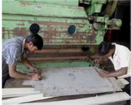
Dimension were marked to cut and bend the Al sheet.
