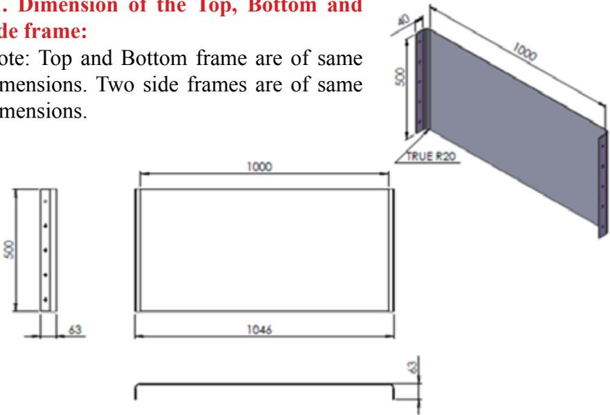
Top and bottom frame dimensions All dimension are in mm
